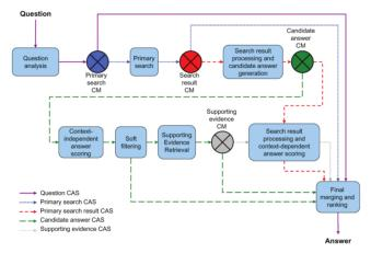
DeepQA architecture (Epstein et al., Making Watson fast). A series of CAS multipliers.
